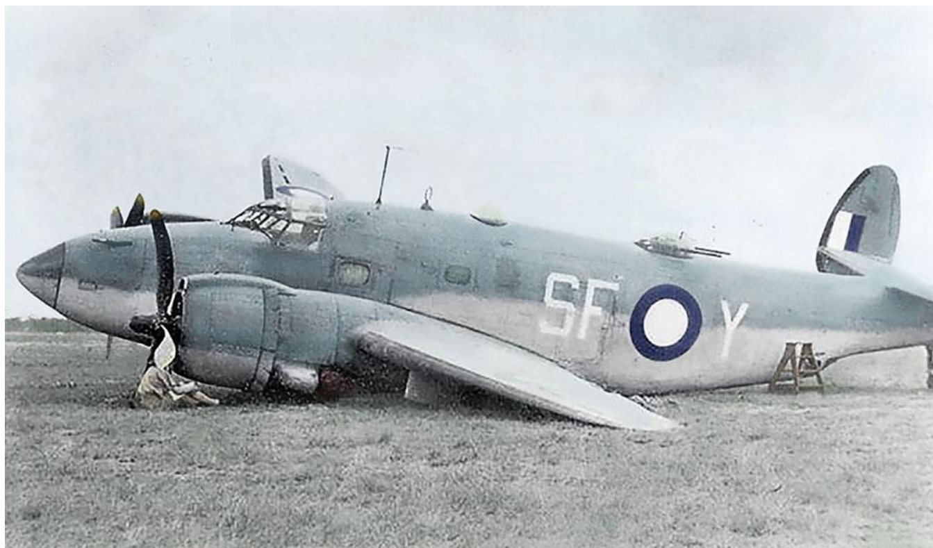
A59-51 SF-Y port undercarriage collapsed in taxi accident at Bundaberg QLD, on 25 OCT 1943
