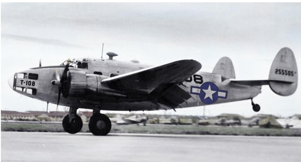
USAAF AT-18A Hudson 42-55505/T-108 navigation trainer without turret
